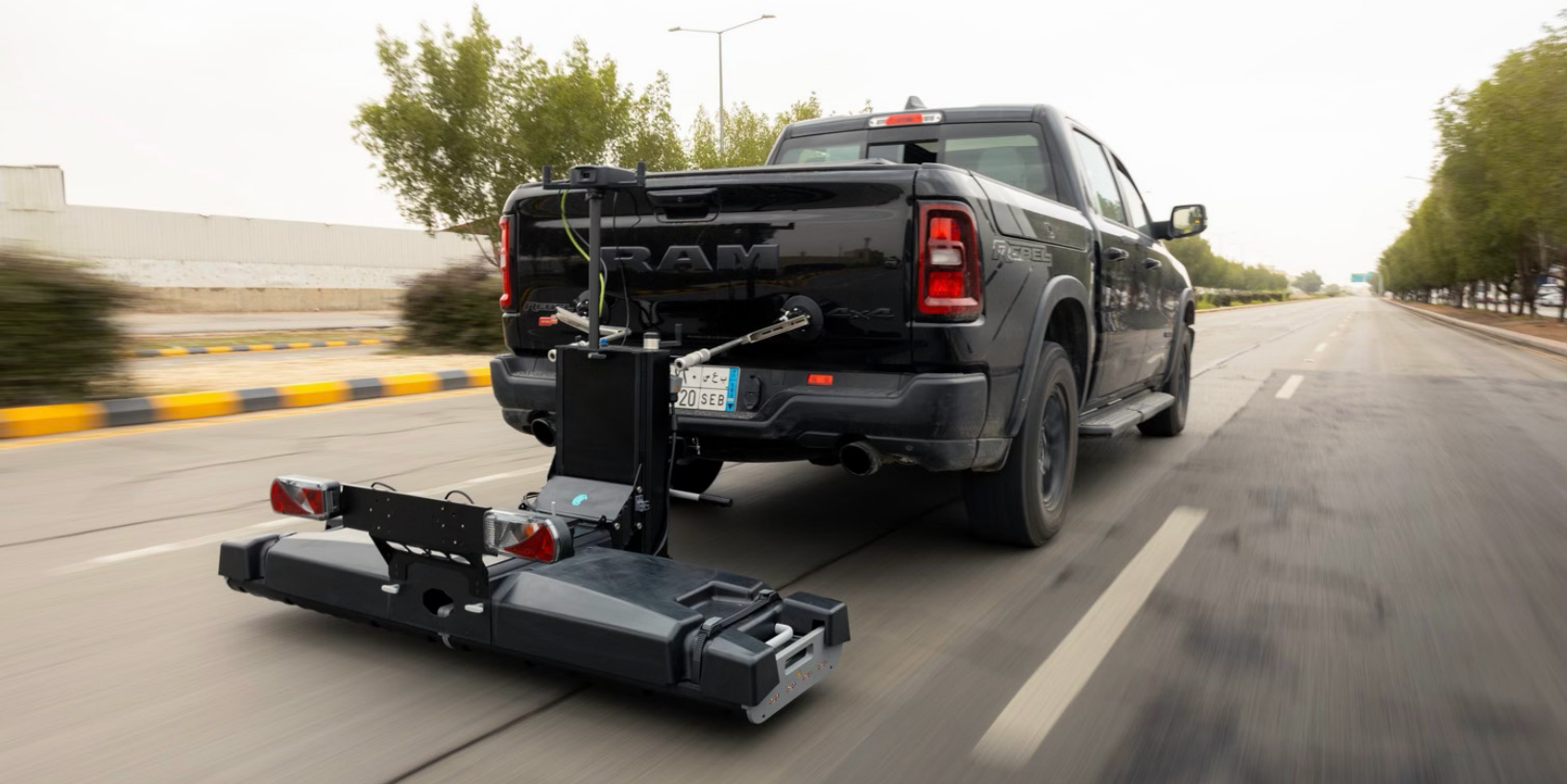
Figure 1. The GM8000 stepped-frequency MCGPR array, shown towed behind a survey vehicle. The same modular array also runs in a push-cart configuration for footpaths and constrained sites.
