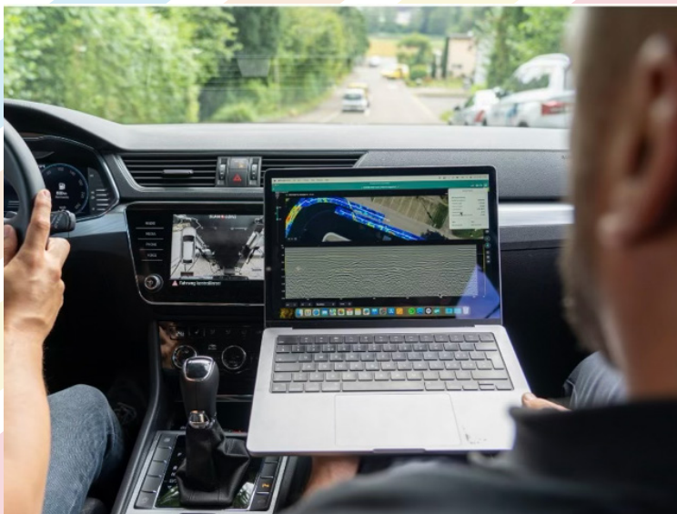
Figure 2. Georeferenced MCGPR data rendered live over aerial imagery during an urban survey. A white trajectory indicates a fixed RTK position; operators verify coverage against satellite and CAD / GIS as-built layers while still on site.
