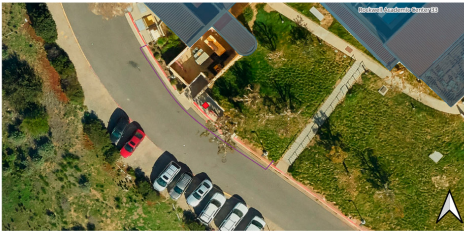
Overlay of the processed utility trench model on a QGIS basemap for geospatial context and alignment with existing site features
