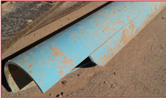
PVC Pipe That was Placed on Rocks
