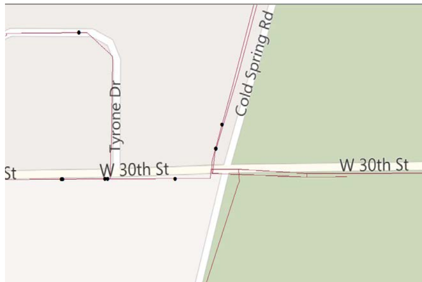
Figure 3.6 Several breaks occurring in a 12 " CI installed in 1945
